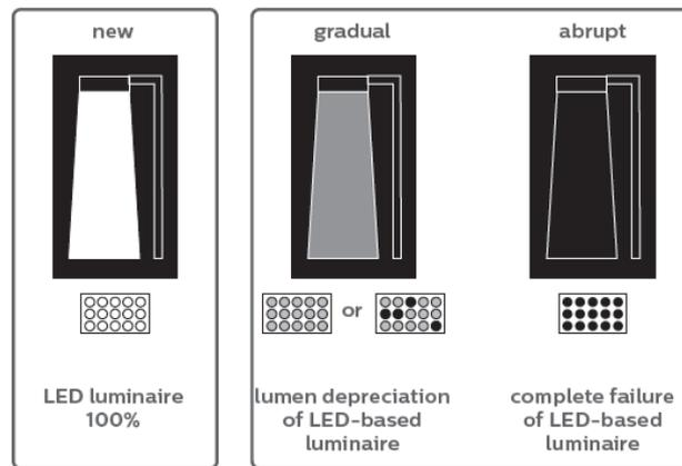
**Fig 1 – Evaluating ‘initial’ and ‘useful lifetime’ performance of LED based luminaires**
